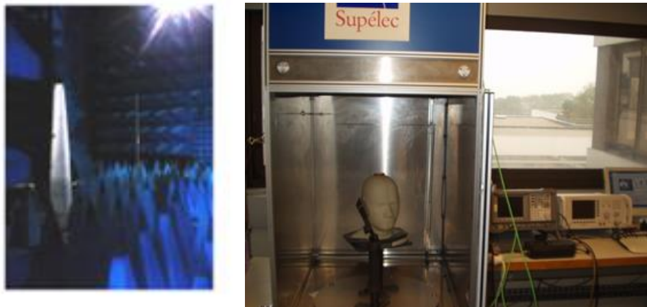
Figure 1.5-i: OTA measurement facilities at CentraleSupélec using anechoic chamber (right) and compact reverberation chamber (left)
