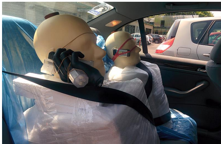
Figure 2.9-i: Outdoor measurement setup for mobility scenario
