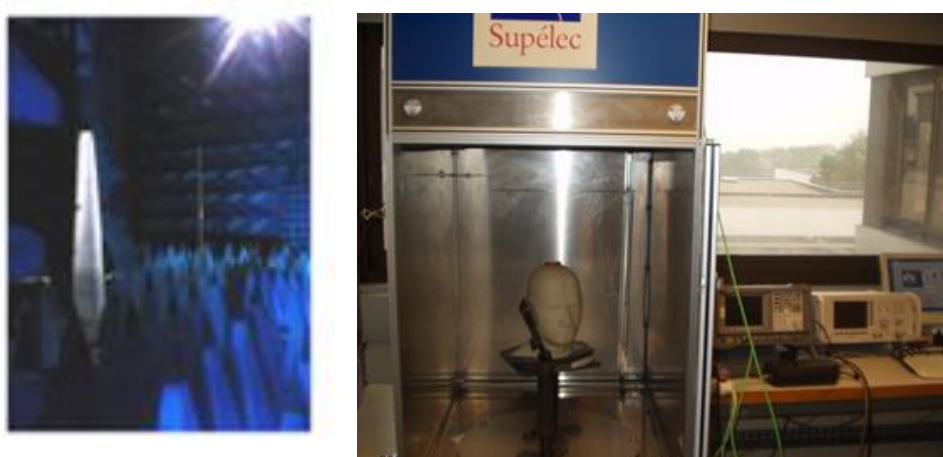
Figure 1.5-i: OTA measurement facilities at CentraleSupélec using anechoic chamber (right) and compact reverberation chamber (left)
