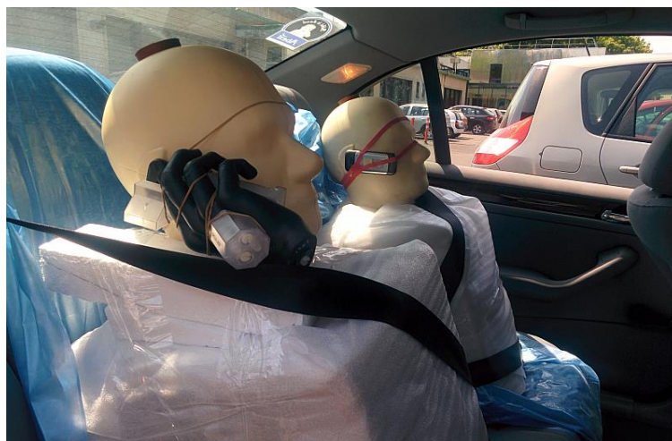
Figure 2.9-i: Outdoor measurement setup for mobility scenario
