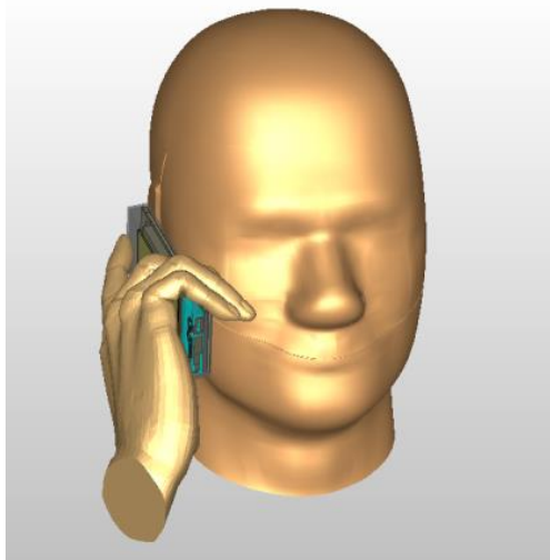
Figure 3.3-i: The numerical representation of the mobile phone placed in the right cheek position against the SAM phantom using a hand phantom
