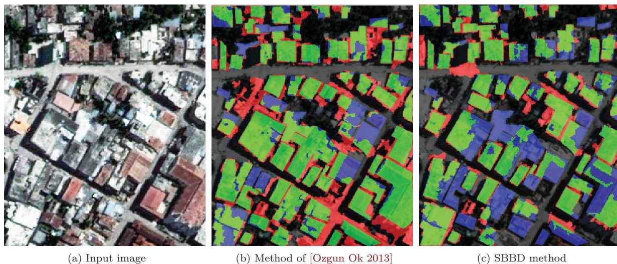
Figure 6.6: Comparisons with method in [Ozgun Ok 2013] on Worldview-2 images of Jacmel dataset.
