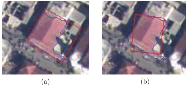
Figure 5.13: Building with protrusion artifact: (a) Building region (whose boundary is delineated by blue line) and its minimum bounding rectangle (red line). (b) Building region and the fitted rectangle estimated by discrepancy method.
