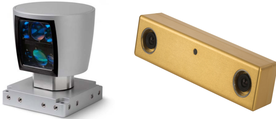
(a) Velodyne high definition Lidar-64 lasers (b) Point Grey research's stereo vision camera systems: Bumblebee2
