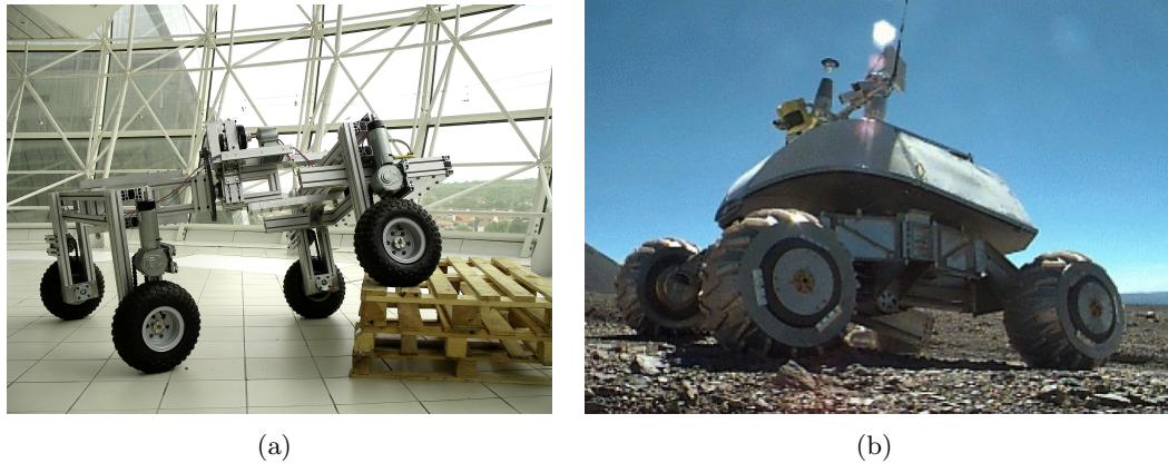
FIGURE 2.7: Wheeled mobile robots: a) OpenWheel: All terrain four wheeled robot [48]; b) Nomad: Four-wheeled robot [180]
