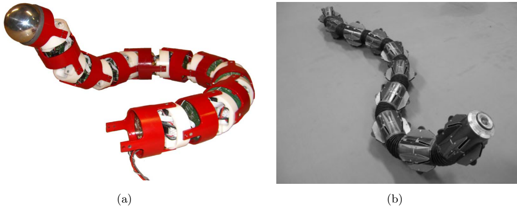
FIGURE 2.5: Crawling mobile robots: a) Aiko: 7kg, 1.5m long, 20 DOF, 2.5 Nm Obstacle-aided locomotion, slidewinding [165]; b) Active Cord Mechanism ACM-R5: 7.5kg, 1.7m long, 80mm diameter Snake propulsion on ground and water [161]
