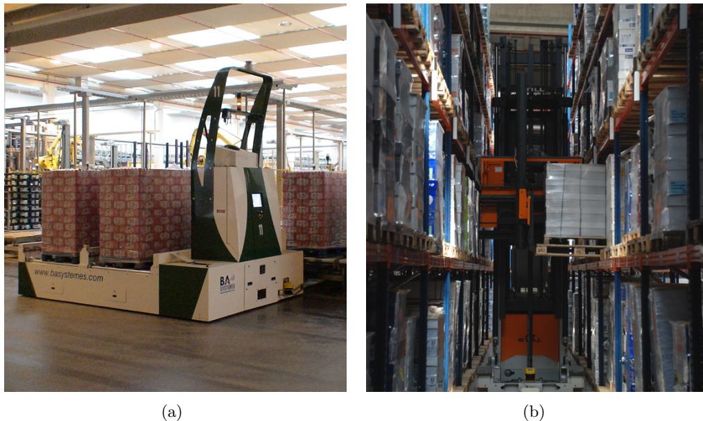
FIGURE 2.9: Industrial robots: a) BA SYSTEMES "Automated Guided Vehicle (AGV)" [157]; b) Duro Felguera "Automatic Storage Retrieval Systems (ASRS)" [81]
