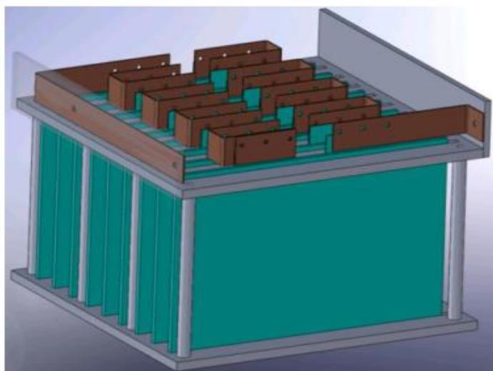
Figure B. 3: Module tampon (100AH, 34V, 500A/200A)
