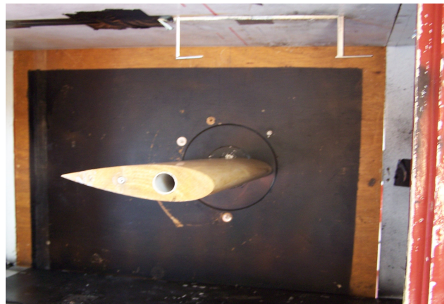
Figure C.3: An NACA 0024 airfoil is mounted in side the wind tunnel.
