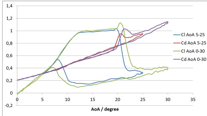
Figure C.8: Lift and drag coefficients for 2 test cases with the same oscillation frequency  $f = 0.3$  Hz, and different oscillation amplitudes.
