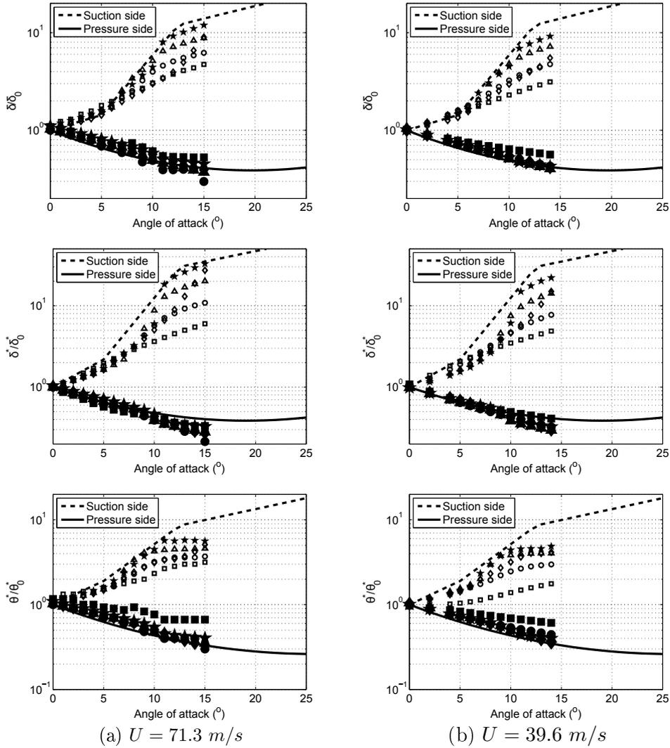
Figure 2.15: Comparison of  $\delta^*$ ,  $\delta$  and  $\theta^*$  calculated by XFOIL for tripped cases at various AoA. Symbol shapes are consistent with Figure 2.14. Empty symbols are for suction side, and filled symbols are for pressure side. Left column consists figures with free stream velocity  $U = 71.3 \text{ m/s}$ , right column consists figures with free stream velocity  $U = 39.6 \text{ m/s}$ . Subscription  $_0$  stands for the corresponding terms at  $0^\circ$  AoA.
