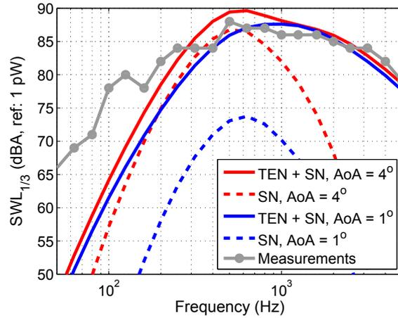
(a) Reference velocity  $U_{ref} = 6 \text{ m/s}$ , pitch angle is  $3^\circ$ , corresponding to AoA of  $1^\circ$ .
