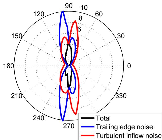
Figure 3.28: Directivity of amplitude modulation by a receiver at 100 m away from the wind turbine for case 2 with  $H = 0$  (neutral atmosphere) when looking from above, and the wind is coming from the left.
