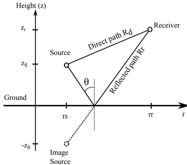
Figure 4.1: Illustration of the image source model with direct and reflected paths.
