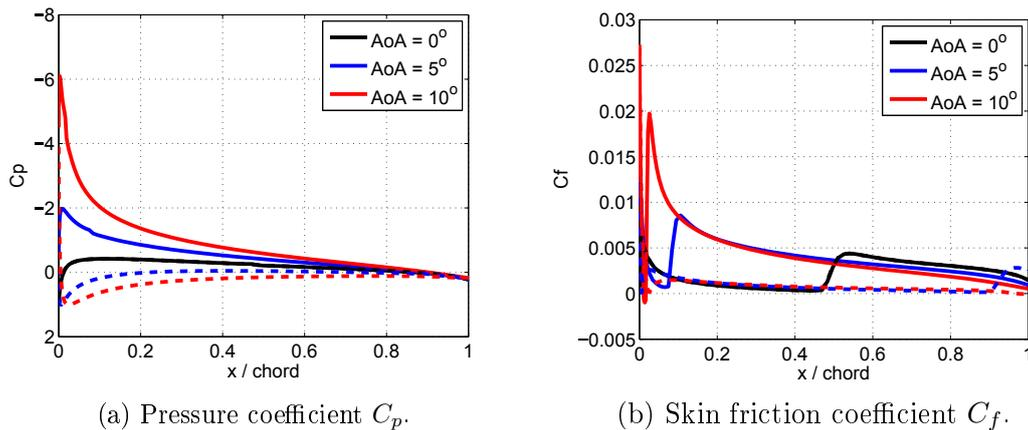
(a) Pressure coefficient  $C_p$ .(b) Skin friction coefficient  $C_f$ .Figure 2.7: Pressure and skin friction coefficients for a NACA 0012 airfoil at a Reynolds number of  $4 \cdot 10^6$ . Solid lines: suction side; dashed lines: pressure side.
