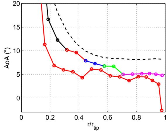
Figure 3.4: Angle of attack along the blade of the 5MW wind turbine calculated by BEM theory. Black dash line: induced velocity is not considered ( $a = a' = 0$ ); color line: induced velocity is considered, and colors corresponds to different profile sections as shown in Figure 3.5; red line: induced velocity is considered and predicted by FAST. Tip loss factor is considered.
