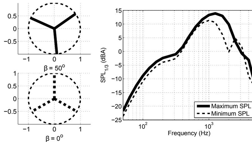
Figure 4.30: Spectra of two blade positions where the maximum and the minimum SPL level are observed for the third octave centered at  $f = 2000$  Hz. Blade rotates clockwise. Observer is at 1000 m crosswind direction. Upper left: blade position when the maximum SPL is produced; lower left: blade position when the minimum SPL is produced.
