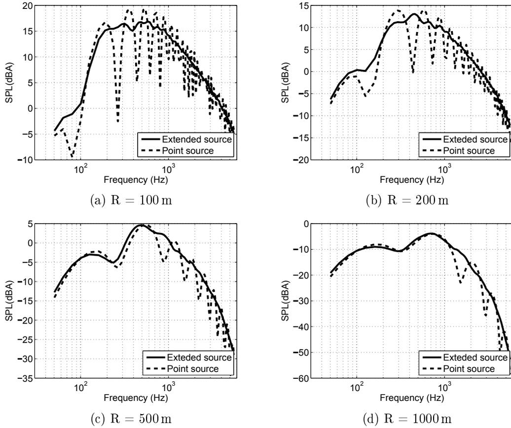
Figure 4.36: Narrowband SPL for point source and extended source calculations at different source-receiver distance in the downwind direction. Solid lines: extended source; dashed line: point source.
