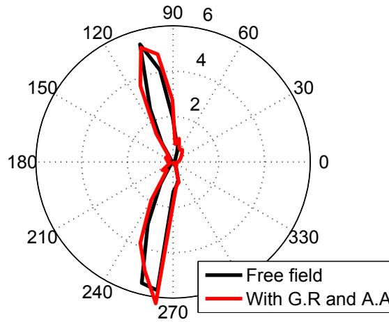
Figure 4.27: Directivity of amplitude modulation strength for free field and for a grassland with consideration of ground reflection and atmosphere absorption. Observer distance is 1000 from the wind turbine.  $\sigma_e = 200kPa \cdot s \cdot m^{-2}$ .
