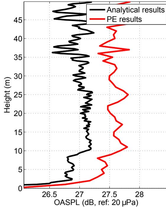
Figure 4.15: Comparison of overall SPL as a function of height for an impedance ground with  $\sigma_e = 200 \text{ kPa} \cdot \text{sm}^{-2}$  between analytical solution and PE results. Observer is 1000 m away in the downwind direction. Blade position parameter  $\beta = 0^\circ$ .
