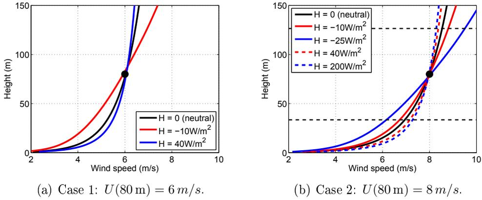
Figure 3.12: Mean wind profiles  $U(z)$  for the atmospheric conditions described in Table 3.3. The minimum and maximum rotor heights are shown using black dashed lines.
