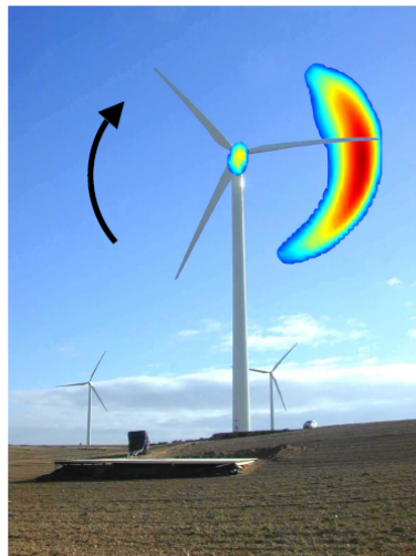
Figure 1.2: Noise source distribution in the rotor plane of a modern large wind turbine, measured about one rotor diameter upwind from the turbine. Taken from [2].
