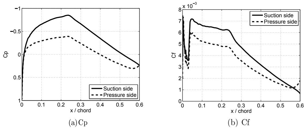
Figure 2.12: Pressure coefficient and skin friction coefficient for NACA64<sub>3</sub>418 airfoil at zero AoA.
