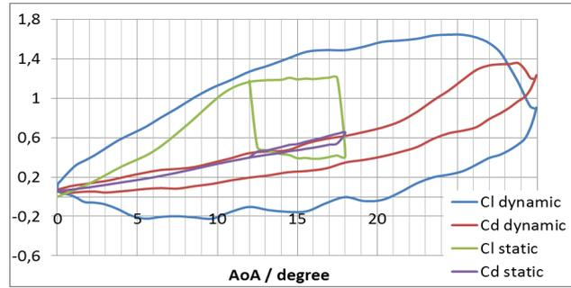
Figure C.6: (Continued) Lift and drag coefficients measured for dynamic stall cases compared to static case. Case 5,  $f = 2.6$  Hz, range of AoA = 0 – 30°.
