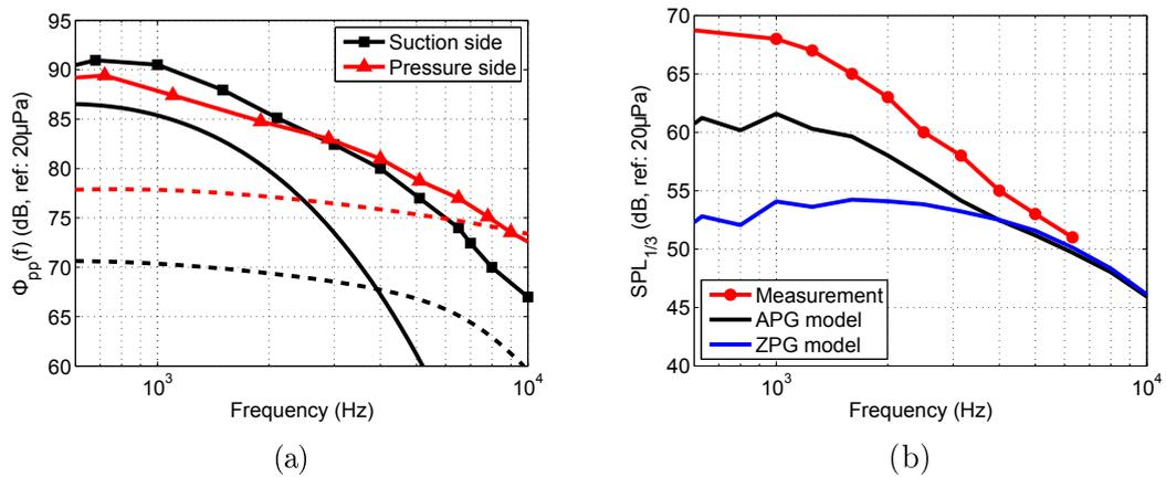
Figure 2.13: (a) Wall pressure spectra on the suction side (black lines) and on the pressure side (red lines) measured by Kamruzzaman *et al.* [12] (symbols) and predicted by APG (solid lines) and ZPG models (dashed lines) models. (b) Third octave band spectra of far-field SPL. Symbols: measurements; black line: APG model applied on suction side, and Goody's ZPG model on pressure side; blue line: ZPG model.
