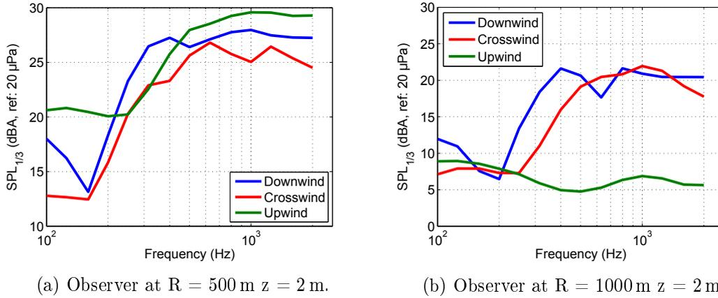
Figure 4.33: Third octave band SPL spectra averaged over blade position  $\beta$  in downwind, crosswind and upwind directions.
