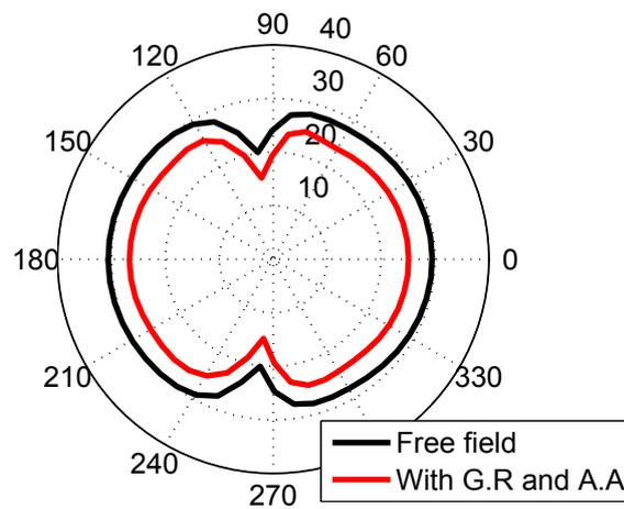
Figure 4.26: Directivity of overall SPL for free field and for a grassland with consideration of ground reflection and atmosphere absorption. Observer distance is 1000 from the wind turbine.  $\sigma_e = 200 \text{ kPa} \cdot \text{s} \cdot \text{m}^{-2}$ .
