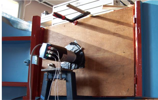
Figure C.2: Rotating system and the aerodynamic balance.
