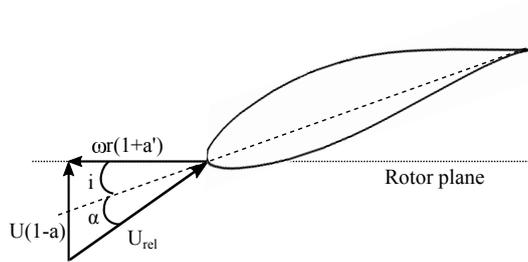
Figure 3.2: Induced velocity in the rotor plane.
