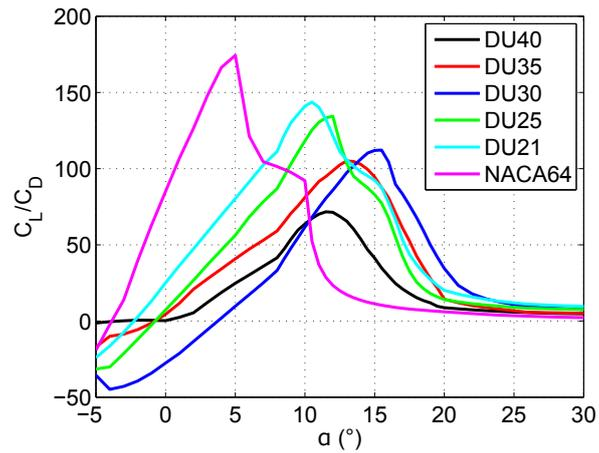
Figure 3.5:  $C_l/C_d$  for all the blade sections mentioned in [15].
