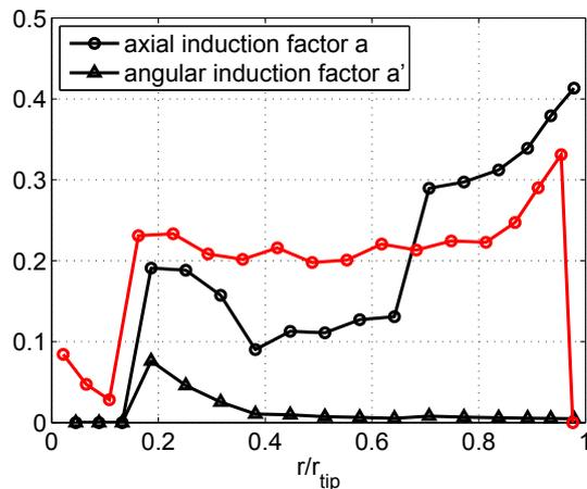
Figure 3.6: Axial and angular induction factors calculated by our BEM code (black lines), and axial induction factor calculated by FAST (red line) for a 5MW wind turbine.
