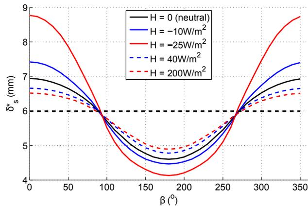
Figure 3.19: Variation of displacement thickness  $\delta_s^*$  on the suction side as a function of blade azimuthal position  $\beta$  for the tip segment for case 2. The thick dashed line corresponds to the reference value with a constant wind profile.
