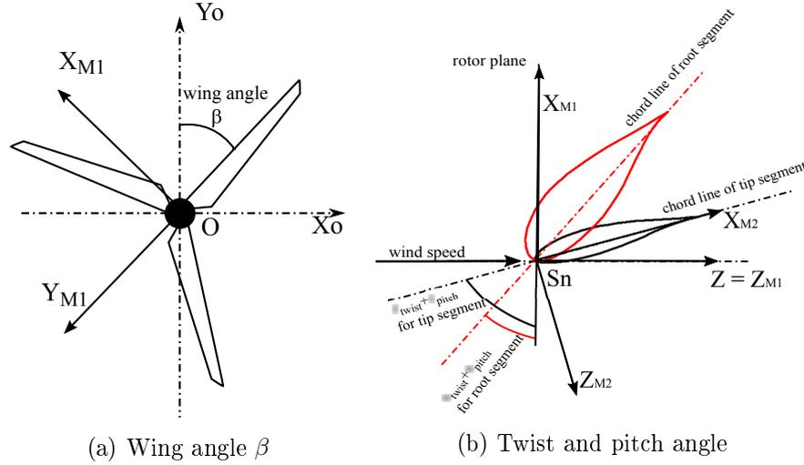
Figure 3.11: Illustration of relative angle during coordinate transfer.
