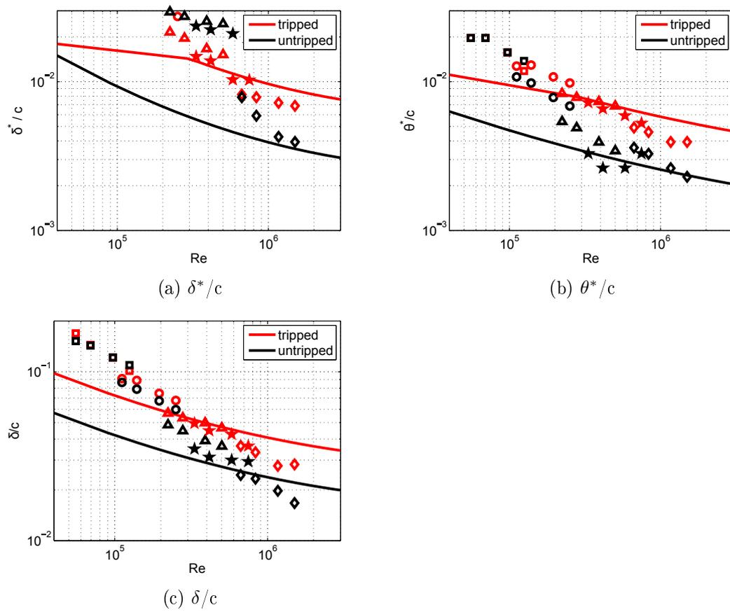
Figure 2.14: Boundary layer parameters calculated with XFOIL (symbols) comparing with empirical curves (lines) given by [1],  $AoA = 0^\circ$ . Symbols represent different chord length:  $\diamond$ , 0.3048m;  $\star$ , 0.1524m;  $\triangle$ , 0.1016m;  $\circ$ , 0.0508;  $\square$ , 0.0254m.
