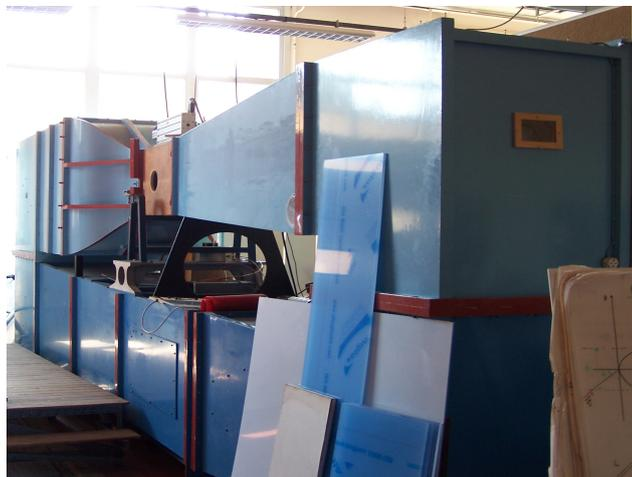
Figure C.1: Closed return wind tunnel at ENSTA ParisTech.
