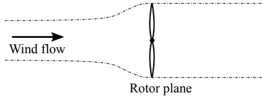
Figure 3.1: Free flow passing through the rotor plane.
