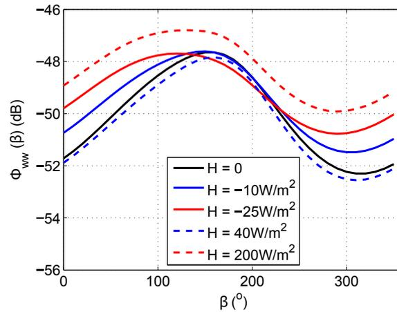
Figure 3.23: Variations of turbulence spectrum  $\Phi_{ww}$  as a function of blade azimuthal position  $\beta$  for the tip segment at 100 Hz and for the various atmospheric conditions corresponding to case 2.
