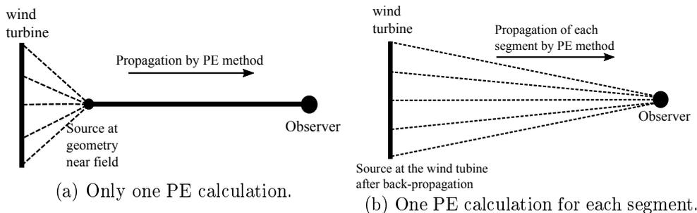
Figure 4.11: Illustration of the two methods considered for the coupling between source and propagation models.
