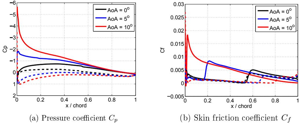
Figure 2.8: Pressure and skin friction coefficients for a NACA 63-415 airfoil at a Reynolds number of  $4 \cdot 10^6$ . Solid lines: suction side; dashed lines: pressure side.
