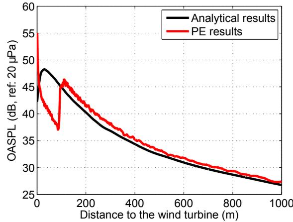
Figure 4.16: Comparison of overall SPL as a function of propagation distance for an impedance ground with  $\sigma_e = 200kPas m^{-2}$  between analytical solution and PE results. Observer is at 2 m height in the downwind direction. Blade position parameter  $\beta = 0^\circ$ .
