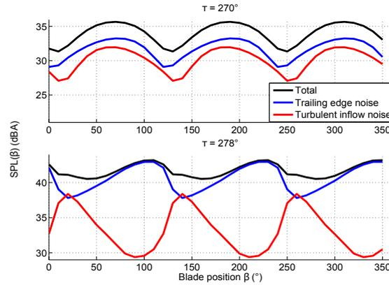
Figure 3.30: Amplitude modulation for trailing edge noise, turbulent inflow noise and for the overall noise at an horizontal angle of  $270^\circ$  (top) and of  $278^\circ$  (bottom) with respect to the wind direction, for case 2 and  $H = 0$ .
