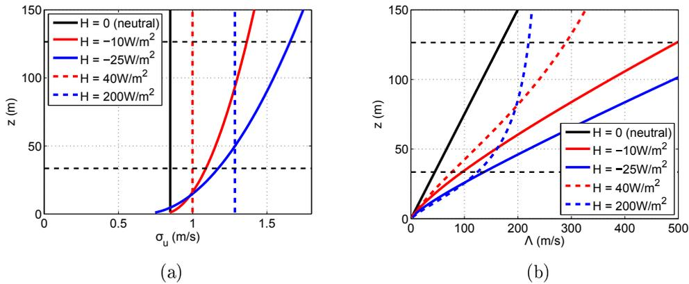
Figure 3.13: (a) Standard deviation of turbulent velocity fluctuations  $\sigma_u$  and (b) integral length scale  $\Lambda$  for a reference velocity of  $U(80\text{ m}) = 8\text{ m/s}$ . The minimum and maximum rotor heights are shown using black dashed lines.
