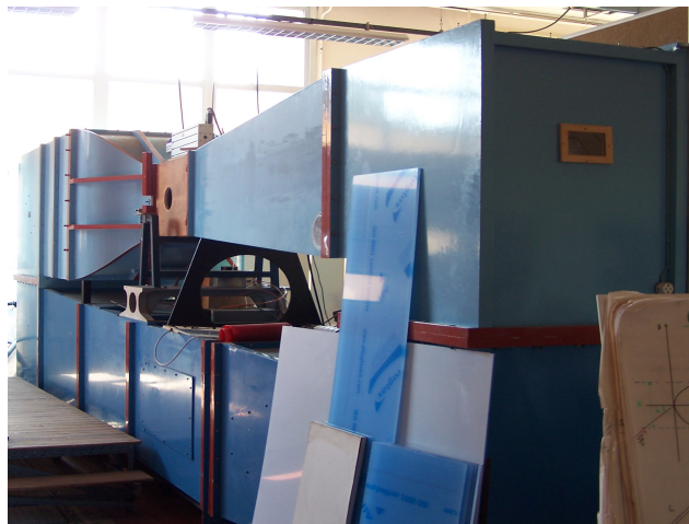
Figure C.1: Closed return wind tunnel at ENSTA ParisTech.
