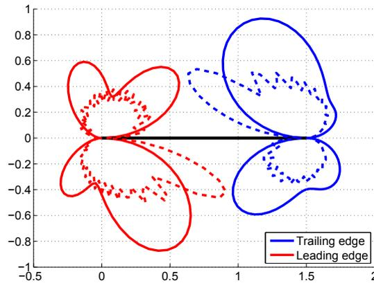
Figure 3.29: Normalized directivity of TE and TI for the tip segment of the blade who is pointing up. Solid lines:  $f = 500\text{ Hz}$ ; dashed lines:  $f = 4000\text{ Hz}$ .
