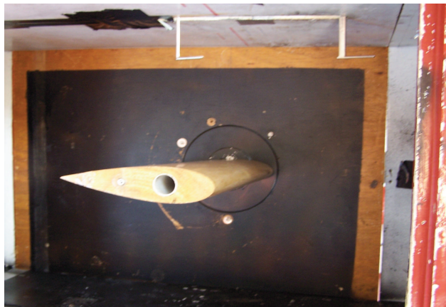
Figure C.3: An NACA 0024 airfoil is mounted inside the wind tunnel.
