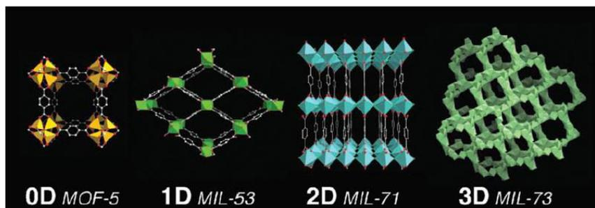
*Figure I-3 : exemples de structures MOF (Metal Organic Framework)
