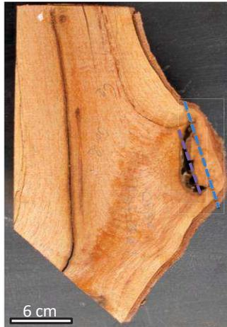
A branch stump in longitudinal section showing stump diameter ( $D_{stump}$ ) (blue line) and shed branch diameter ( $D_{sb}$ ) (purple line).
