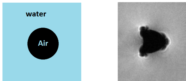
Figure 1.2.12: Demonstration of the effect of magnetic susceptibility of a cylindrical water/air interface; distortions and intensity loss in the GRE acquired image: B_0 = 7\text{T} , \text{TR} / \text{TE} = 500/15\text{ ms} , matrix = 256 \times 256 [Belaroussi, 2005].
