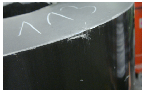
(c) Observation of long fibrils at the end of the compaction step at the surface of the green part
