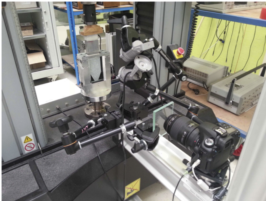
Figure 3.21: V tool inside the testing machine and with the picture acquisition set up
