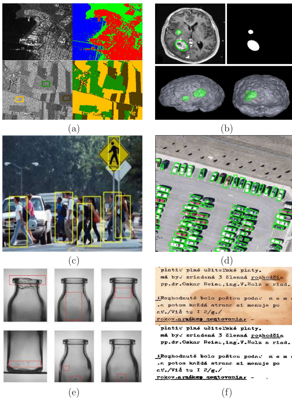
FIGURE 1.2: Some popular image segmentation applications. (a) SAR images for remote sensing. (b) MRI brain tumor detection and segmentation. (c) Pedestrian detection. (d) Object detection (cars). (e) Defect detection for glass bottles. (f) Document analysis and recognition.
