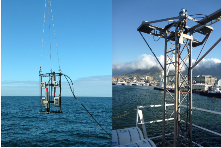
Figure 3.10: Picture of the in-water TriOS RAMSES system deployed in a cage during the MV1102 measurement campaign (left) and the deck sensor for the normalization of the in-water radiometric measurements to variations in illumination (right).
