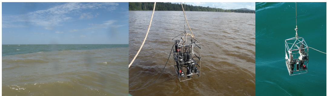
Figure 1.1: Different water colours reflect variations in in-water constituents and concentrations. Turbid plume penetrating ocean waters dominated by phytoplankton along the coastal region of French Guiana (left). In situ water sensors over brownish water masses dominated by high SPM concentrations in French Guiana (centre) and over phytoplankton dominated greenish water masses in the Southern Atlantic Ocean (right).
