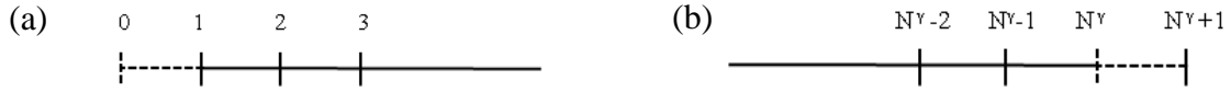
Figure IV. 7: Schematic of the virtual points at the (a) left and (b) the right boundaries of the calculation cell.
