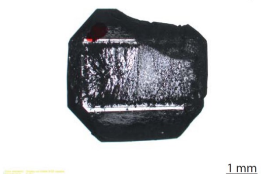
AG13-04 500 °C-200 MPa-NaOH 1M -114 days
