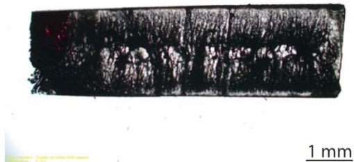
AG13-01 500 °C-200 MPa-NaOH 2M -21 days
