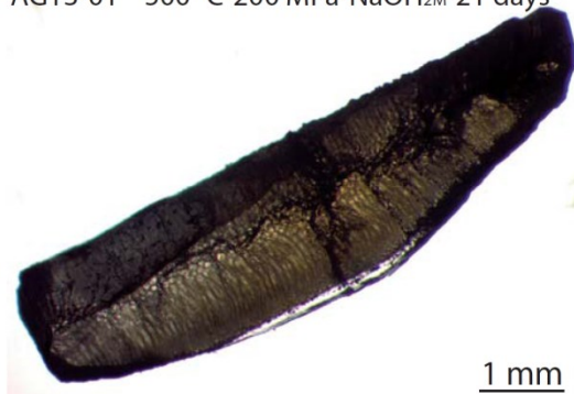
AG13-06 300 °C-200 MPa-NaOH 1M -114 days
