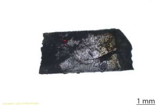
AG13-03 500 °C-200 MPa-NaOH 1M -114 days
