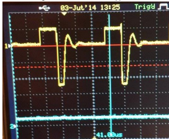
Figure B. 6 Waveforms of the Buck-Boost's inductor voltage (yellow) and SSHI series recuperated energy (blue)
