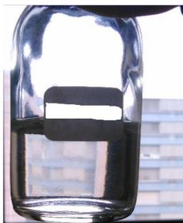
**Figure 5.1:** Picture of ZnO NPs synthesized by the hydrolysis of  $\text{ZnEt}_2$  with a mixture of PAAH and PAANa with the ratio of 50:50 in volume, the concentration of 0.63 wt% and the reaction time of 1h.
