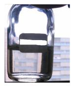
*Figure 5.1*: Picture of ZnO NPs synthesized by the hydrolysis of  $ZnEt_2$  with a mixture of PAAH and PAANa with the ratio of 50:50 in volume, the concentration of 0.63 wt% and the reaction time of 1h.
