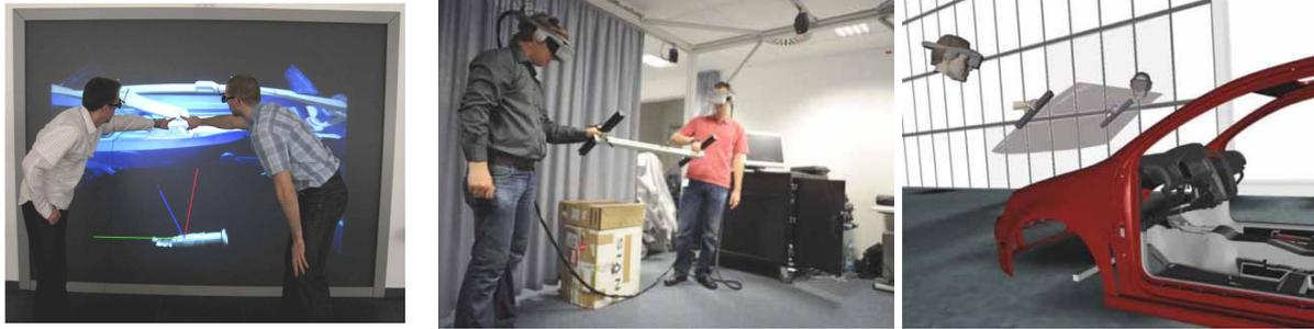
(a) Direct user interaction with deictic gestures (Simon, 2005). 2009a). (b) A windshield assembly task using tangible interface (Salzmann et al., 2009a).
