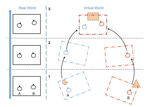
Figure 5.11 – An example of collaborative mode switching: users pass from individual mode to consistent mode (from phase 1 to 3). Users' *stages* are represented by dotted rectangles.
