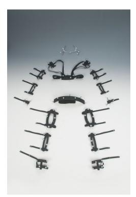
Figure B.2 – The ART-Human Body Tracking Suit by Advanced Realtime Tracking GmbH.
