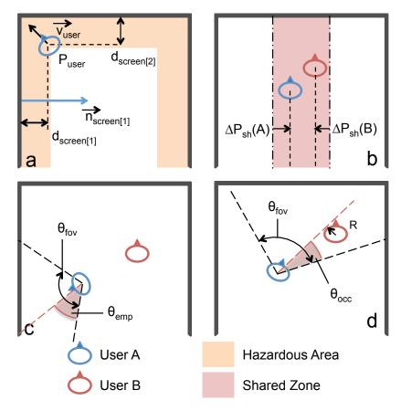
Figure 4.5 – (a) The hazardous area. (b) User's penetration  $\Delta P_{sh}(t)$  in the shared zone. (c) Illustration of seeing empty screen angle  $\theta_{emp}(t)$  and (d) the occlusion angle  $\theta_{occ}(t)$ .
