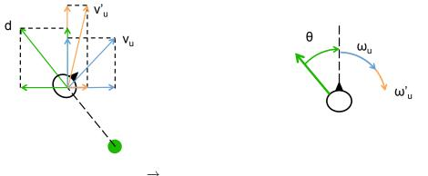
(a) Velocity vectors are scaled by  $\vec{d}$ . (b) Angular velocity is scaled by  $\theta$ .
