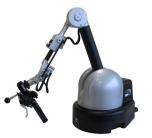
(b) The Virtuose 6D haptic arm © Haption.
