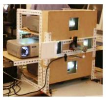
(a) The two-user Responsive Workbench (Agrawala (b) Two-user active separation with four projectors et al., 1997). (Froehlich et al., 2004).
