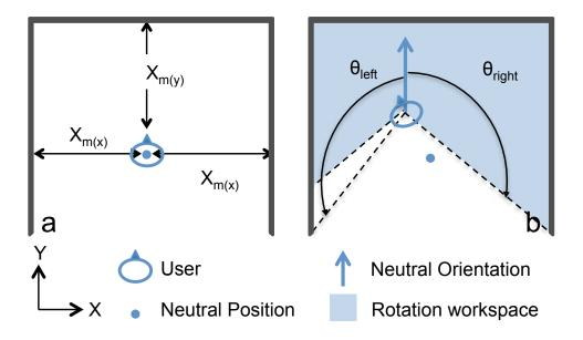
Figure 4.2 – a) The maximum available workspace  $X_m$  can have different values on x and y axis. b) User's rotational workspace is defined by  $\theta_{max}$  on both sides of the neutral orientation.
