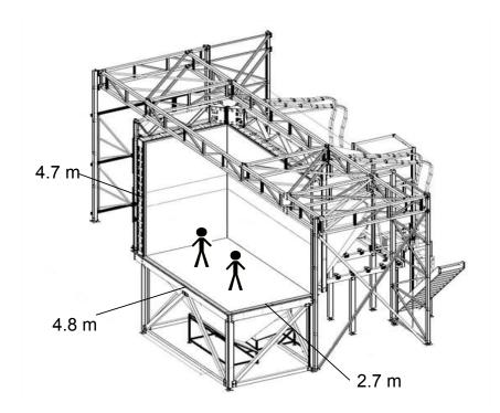
Figure B.1 – The Evolutive Virtual Environment (screen on the right-hand side is not shown in the figure).
