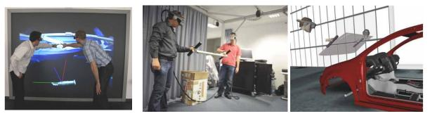
(a) Direct user interaction with (b) A windshield assembly task using tangible interface (Salzmann et al., deictic gestures (Simon, 2005). 2009a).
