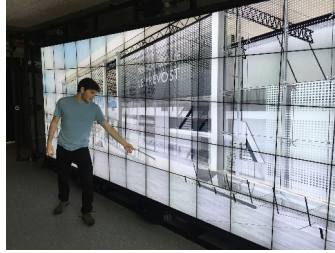
(b) Large image wall composed of high resolution touch screens (WILDER, in|situ|, LRI).
