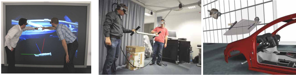
(a) Direct user interaction with deictic gestures (Simon, 2005). 2009a). (b) A windshield assembly task using tangible interface (Salzmann et al., 2009a).
