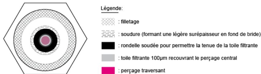
Figure 4.2: Bride – cellule type A
