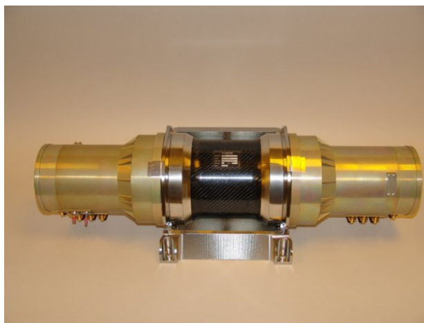
FIGURE 1.13: One of the NaI detectors. Credit: NASA/Fermi
