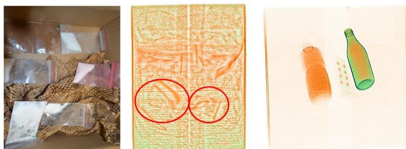
Figure I.7 : Photo and X-ray images of parcels with organic content: powder and liquid.
