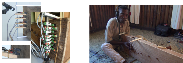
Figure 4.3 – Photos of the set-up installation, where all optical sensors are fixed on a vertical bar along the strings, and also this MCSS in condition of playing
