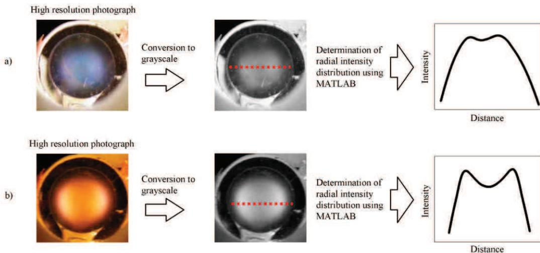
Figure 55. The procedure used to determine the distribution of intensity of light emitted by the discharge. a) discharge maintained in a  $\Phi 5 \times 5$  mm 40 Torr cell with 8 mW of absorbed power. b) The same discharge at 85 mW of absorbed power.
