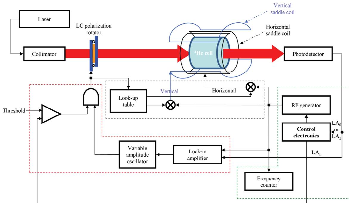
Figure 90. Block scheme of the isotropy-providing system.
