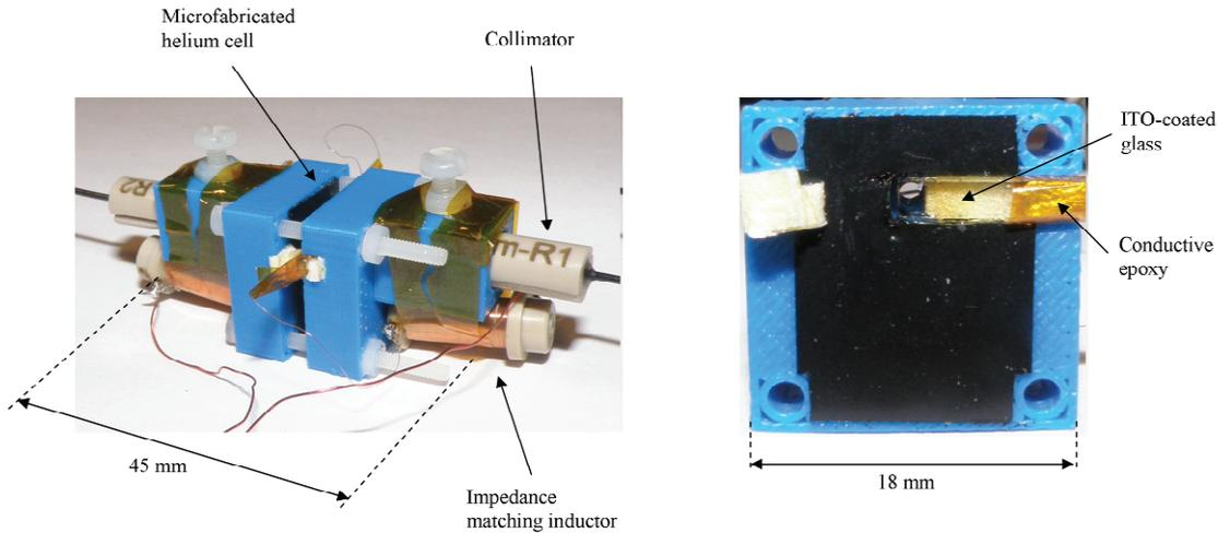
Figure 112. Polymer mount dedicated for absorption measurements in microfabricated helium cells.
