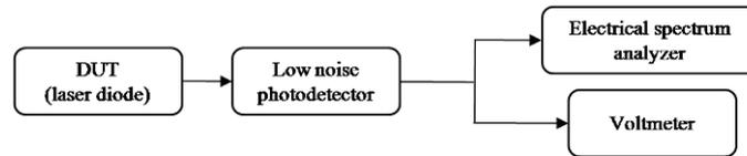
Figure 71. RIN measurement. DUT – Device Under Test.
