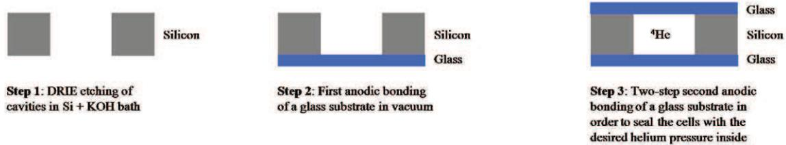
Figure 106. Processing steps used to prepare the microfabricated helium cells.
