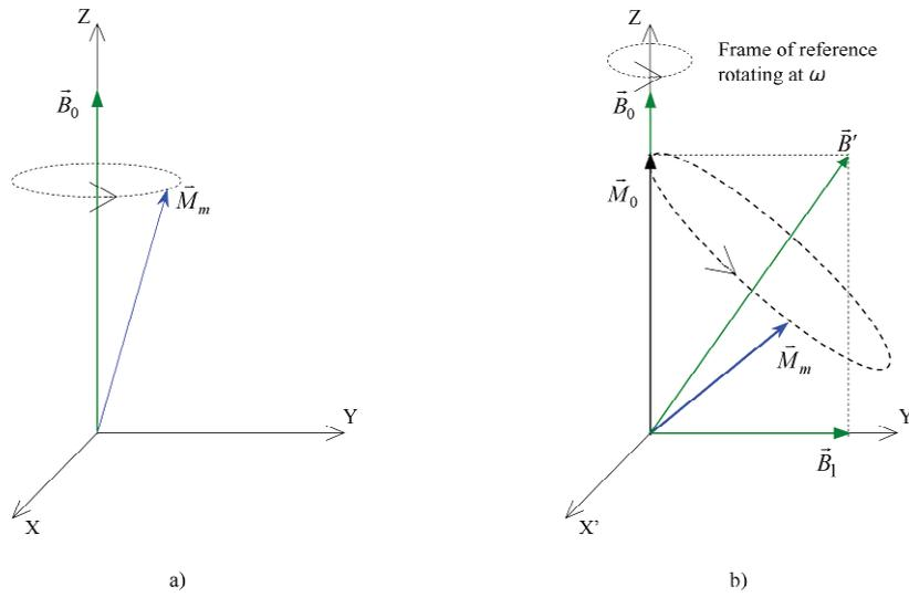
Figure 3. a) Larmor precession. b) Magnetic moment subjected to a constant DC magnetic field  $B_0$  and a rotating RF magnetic field  $B_1$  presented in a frame of reference rotating at an angular frequency  $\omega$  [4].
