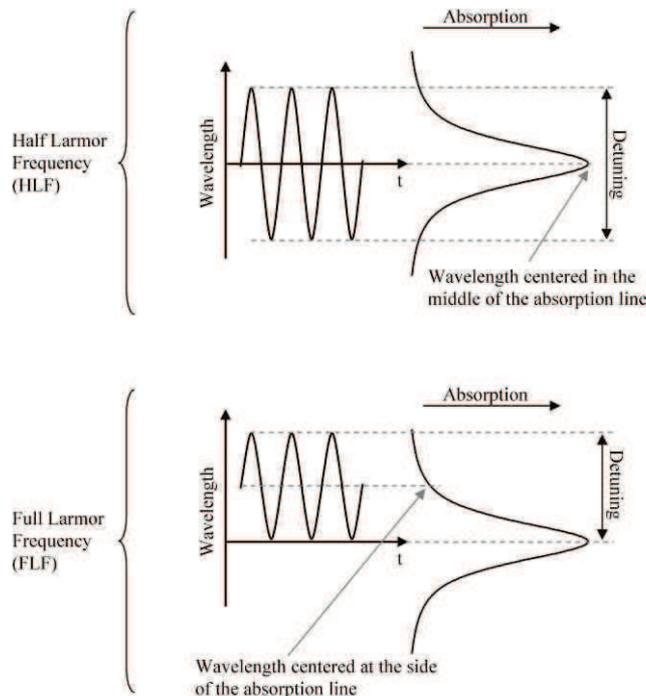
Figure 70. Frequency modulation schemes - Half Larmor Frequency and Full Larmor Frequency. Based on [24].
