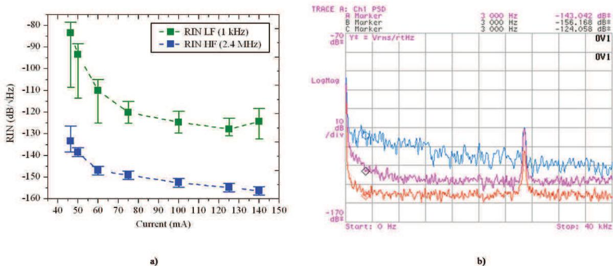
Figure 75. a) RIN noise as a function of current during a stable period. Diode EYP-DFB-1083, S/N: 645. b) Noise characteristics measured with a spectrum analyzer in the arrangement from Fig. 71 without an optical isolator (pink curve). The “jump” in the characteristic - blue curve. The orange curve is the noise of the measurement chain.
