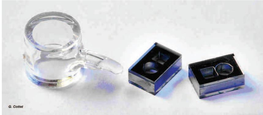
Figure 107. Microfabricated helium-4 cells compared to a miniature  $\Phi 5 \times 5$  mm glassblown cell.
