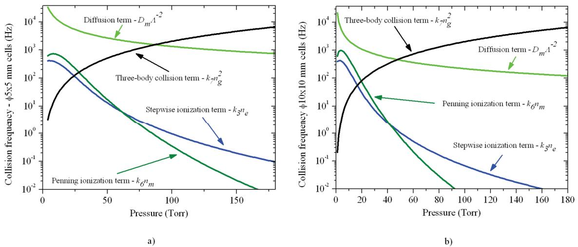
Figure 61. Contributions of four metastable atom destruction mechanisms to the value of the collisional relaxation time calculated by the numerical model. a)  $\phi 5 \times 5$  mm cells. b)  $\phi 10 \times 10$  mm cells.
