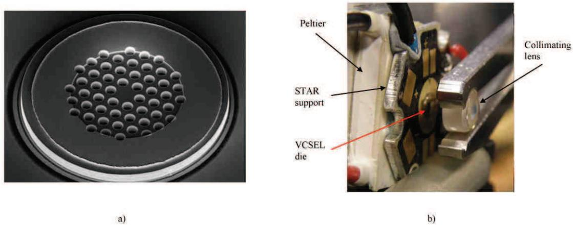
Figure 80. Developed VCSEL laser from the second batch. a) Structure; b) Chip mounted on an optical bench.
