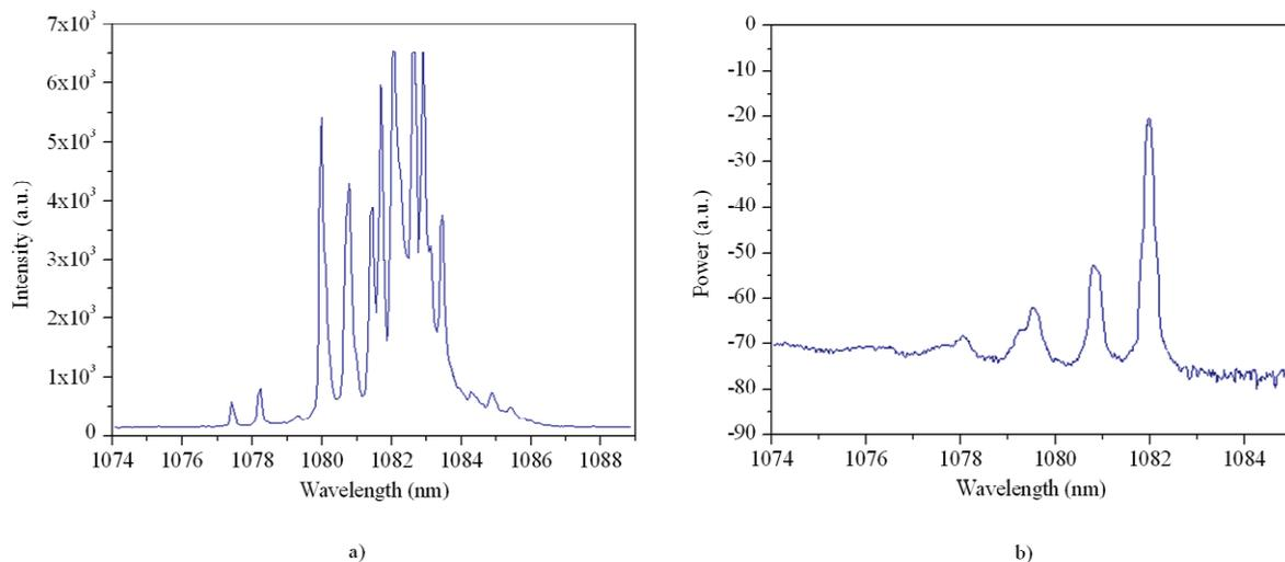
Figure 79. Emission spectra of the developed VCSELS. a) First batch. b) Second batch.
