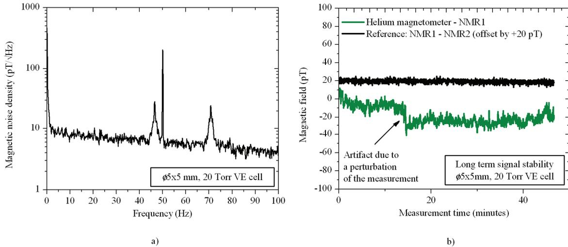
Figure 94. Results obtained with the  $\Phi 5 \times 5$  mm 20 Torr VE cell. a) Magnetic noise density. b) Long term stability.
