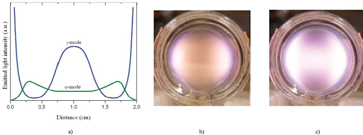
Figure 43. a) Light intensity distribution in  $\alpha$  and  $\gamma$ -modes, data from [26]. b)  $\alpha$ -mode discharge in a 12 Torr 1x1 cm cell at about 200 mW of forward HF power. c)  $\gamma$ -mode discharge in a 12 Torr 1x1 cm cell at about 600 mW of forward HF power.
