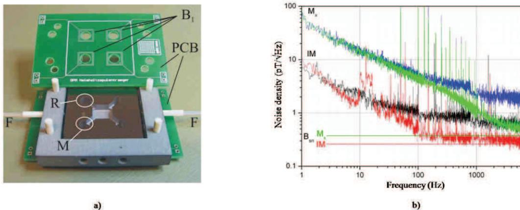
Figure 16. a) Sensor developed at IPHT [17]. b) Comparison between M<sub>x</sub> and Bell-Bloom IM type operation [17]. Red and green traces illustrate a gradiometer mode – subtraction of signals obtained with both cells.
