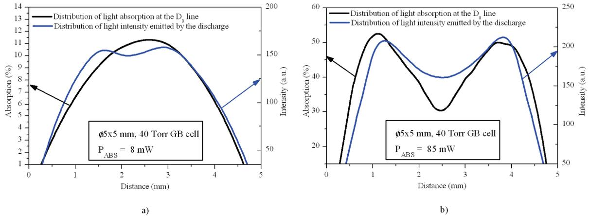
Figure 56. Comparison between the profile of metastable density and the distribution of light emitted by the discharge for a  $\phi 5 \times 5$  mm 40 Torr cell. a) 8 mW of absorbed power. b) 85 mW of absorbed power.
