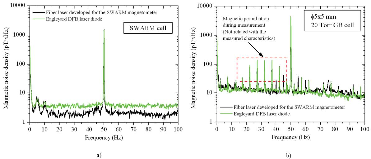
Figure 78. Comparison of noise spectral density of a diode-pumped and fiber laser-pumped magnetometer. a) Measurement done with the SWARM helium cell. b) Measurement done with the  $\Phi 5 \times 5$  mm 20 Torr GB cell.
