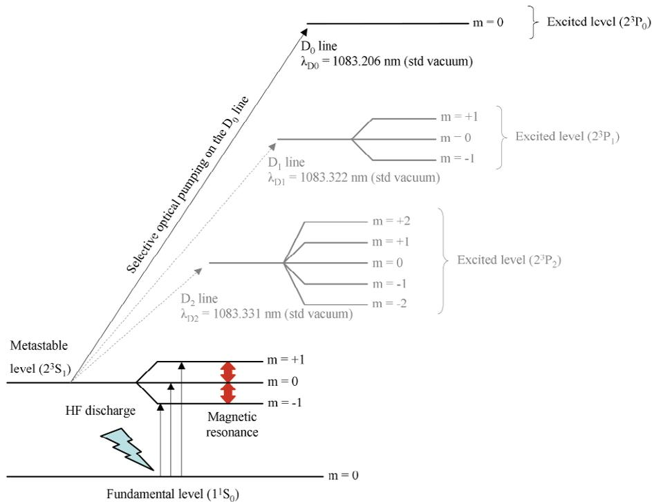
Figure 2. Helium-4 energy band diagram. Not to scale.
