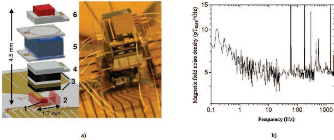
Figure 15. a) Structure of the NIST’s M<sub>x</sub> magnetometer [16]. b) Noise density of the presented magnetometer [16].
