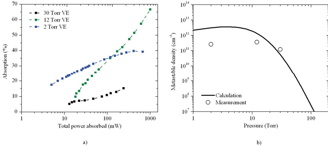
Figure 50. Absorption measurement results  $\Phi 10 \times 10$  mm cells. a) Absorption as a function of power absorbed by the discharge. Data points connected for clarity. b) Values of metastable density at the extinction limit as a function of pressure. Solid curve – issued from the previously described model for 4 mW of power dissipated into the discharge.
