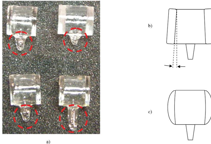
Figure 104. a) Four sample  $\Phi 5 \times 5$  mm helium cells, presenting different geometries of the tip (marked red). b) Angular misalignment between the optical faces of the cell. c) Distortion of the optical faces.
