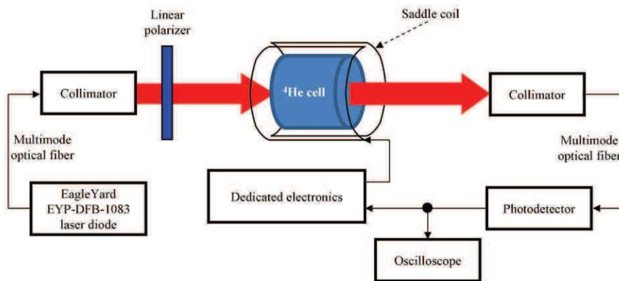
Figure 76. Measurement of sensitivity of a diode-pumped magnetometer.
