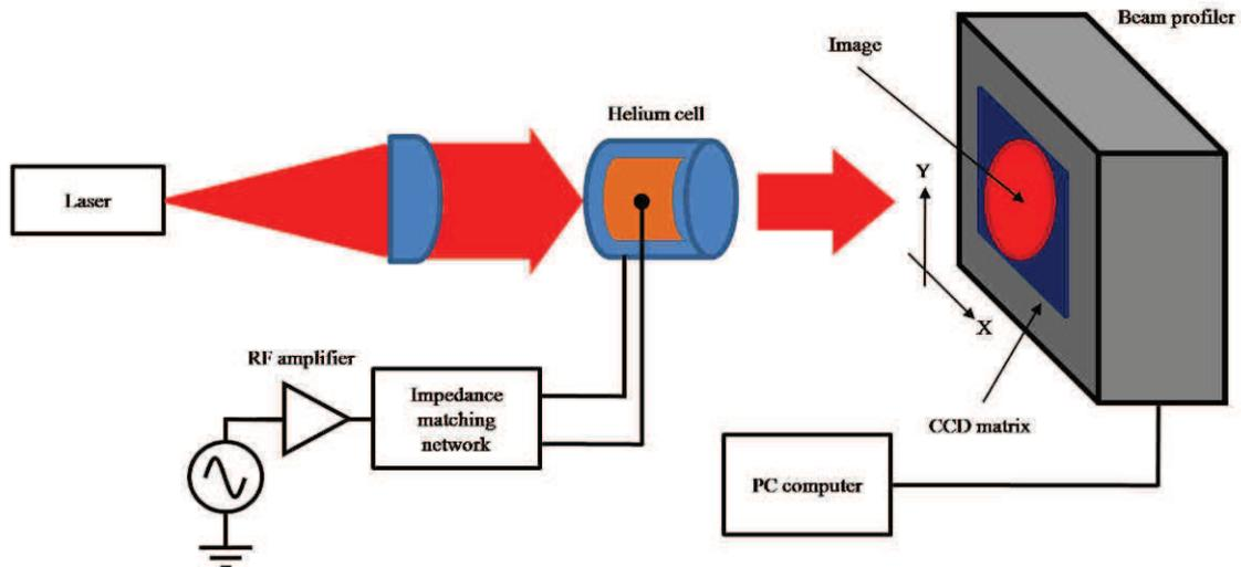
Figure 52. Metastable density profile measurement setup.
