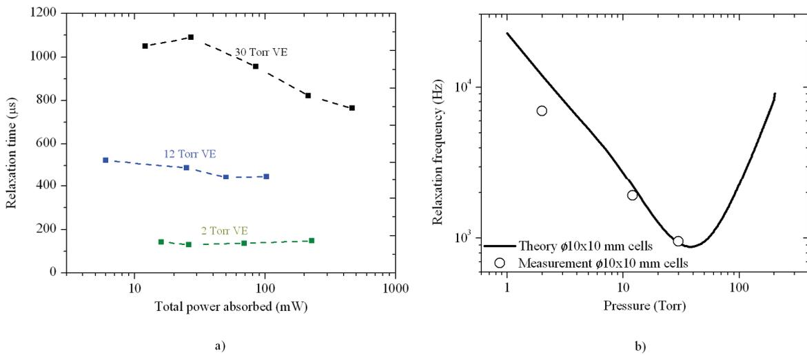
Figure 59. a) Relaxation time measured in the afterglow of discharges in three  $\Phi 10 \times 10$  mm VE cells. Data points connected for clarity. b) Values of relaxation frequency at the extinction limit as a function of pressure. Solid curve – issued from the previously described model for 4 mW of power dissipated into the discharge.
