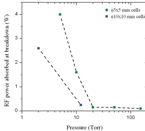
Figure 42. Power absorbed ( $P_{\text{abs}} = P_{\text{Forward}} - P_{\text{Reflected}}$ ) by the matching network of the magnetometer at breakdown ( $f_{RF} \approx 20$  MHz). Data points connected for clarity.
