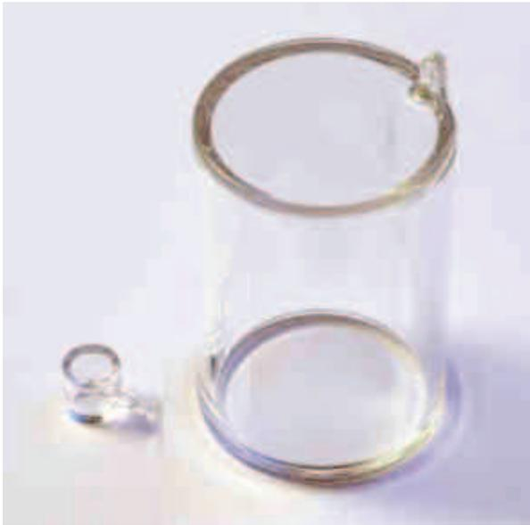
Figure 22. Φ5x5 mm glassblown cell compared to the cell used for the SWARM project (Φ30x45 mm).
