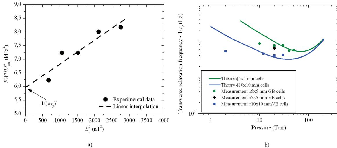
Figure 65. a) Example of a linear interpolation of the measured resonance linewidths.  $\phi 5 \times 5$  mm 30 Torr cell from GB. b) Transverse relaxation frequencies, compared with theory.
