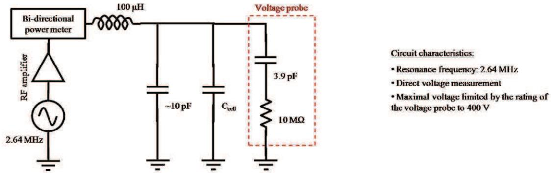
Figure 35. Impedance matching network used for the breakdown voltage measurement at 2.64 MHz.
