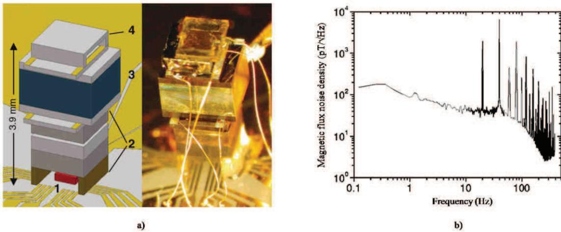
Figure 14. a) Structure of the NIST's CPT magnetometer [3]. b) Noise density of the presented magnetometer [3].
