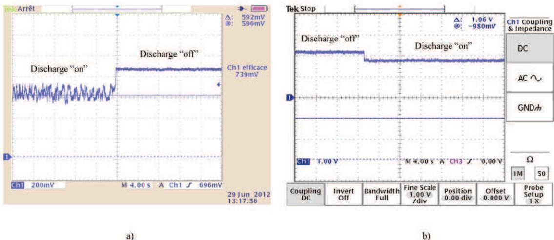
Figure 77. Noise in the output optical signal observed with an oscilloscope. a) without an optical isolator, b) with an optical isolator.
