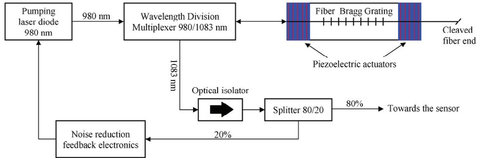
Figure 74. Fiber laser developed for the SWARM project.
