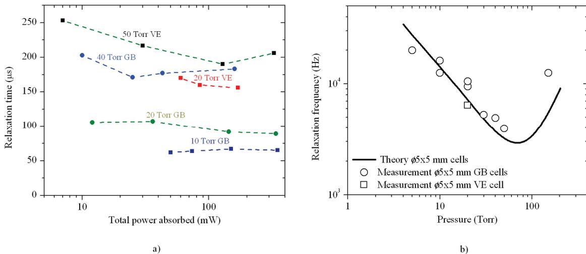
Figure 60. a) Relaxation time measured in the afterglow of discharges in  $\Phi 5 \times 5$  mm cells. Data points connected for clarity. b) Values of relaxation frequency at the extinction limit as a function of pressure. Solid curve – issued from the previously described model for 5 mW of power dissipated into the discharge.
