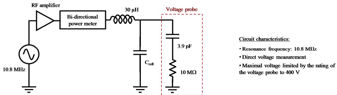
Figure 37. Impedance matching network used for the breakdown voltage measurement at 10.8 MHz.
