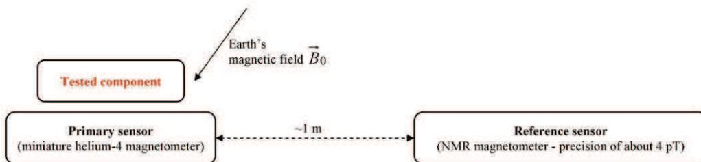
Figure 101. The gradiometer configuration used during the measurement.
