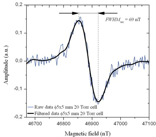
Figure 64. Sample resonance curve for the 20 Torr  $\Phi 5 \times 5$  mm VE cell.
