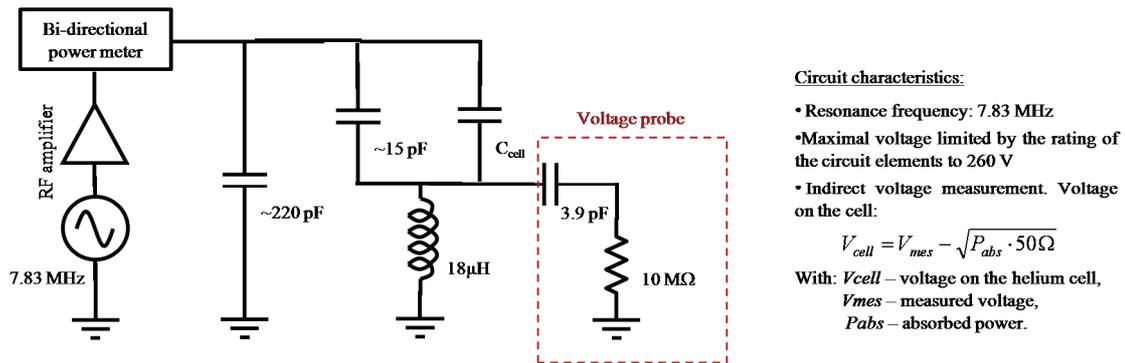
Figure 36. Impedance matching network used for the breakdown voltage measurement at 7.83 MHz.
