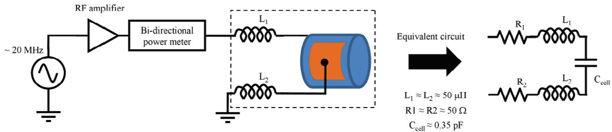
Figure 27. Impedance matching network for the miniature magnetometer.
