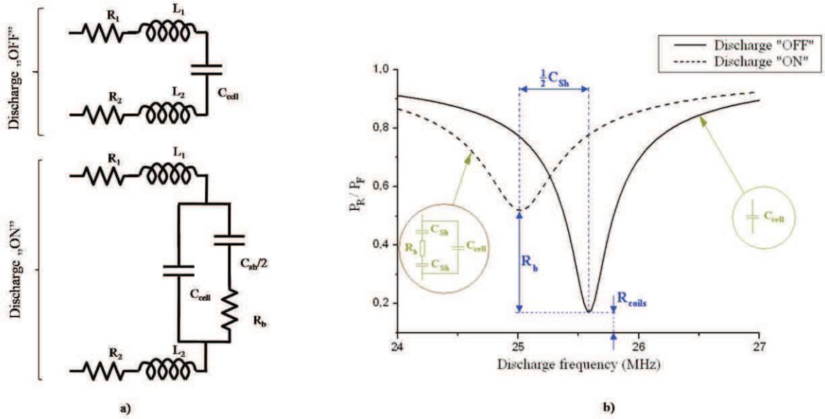
Figure 28. a) Equivalent circuits before and after discharge ignition. b) The ratio of reflected to forward power ( $P_R/P_F$ ), measured with a bidirectional power meter as a function of frequency.
