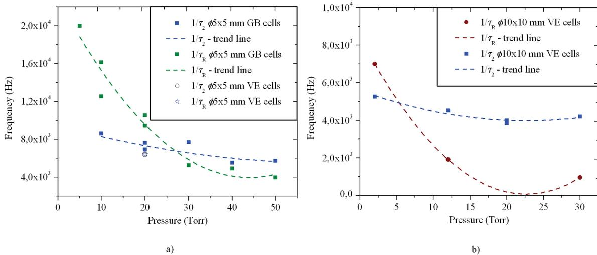
Figure 66. Comparison of transverse and collisional relaxation frequencies. a)  $\Phi 5 \times 5$  mm cells. b)  $\Phi 10 \times 10$  mm cells.
