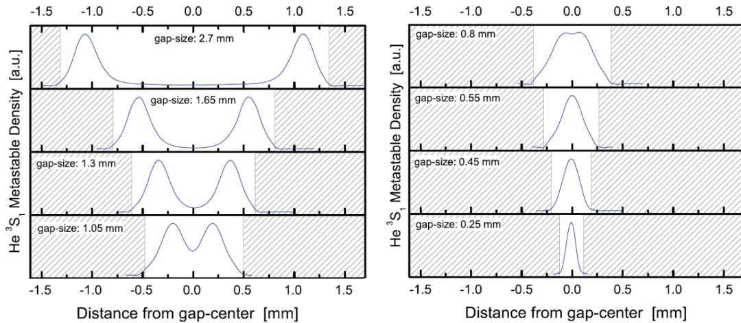
Figure 51. Metastable density distribution in an atmospheric pressure He/O<sub>2</sub>.N<sub>2</sub> plasma for various electrode separation (gap-size) values [45].
