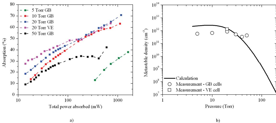
Figure 49. Absorption measurement results  $\Phi 5 \times 5$  mm cells. a) Absorption as a function of power absorbed by the discharge. Data points connected for clarity. b) Values of metastable density at the extinction limit as a function of pressure. Solid curve – issued from the previously described model for 5 mW of power dissipated into the discharge.
