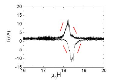
Figure 4.1: Pulsed magnetic field measurement of the current (black) near the field of disappearance of the cycloidal order. Integrating the current leads to a polarization change close to  $10nC/cm^2$ .
