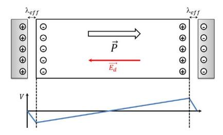
Figure 1.6: Schematic of a metal/ferroelectric/metal structure in capacitor configuration. The imperfect screening of the polarization charges leads to a depolarizing field  $\mathbf{E}_{\mathbf{d}}$  which in turn influence the electric fields at the interface.
