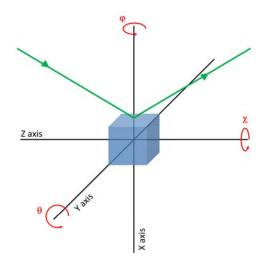
Figure 3.3: Schematic representation of the diffractometer characteristic angles.
