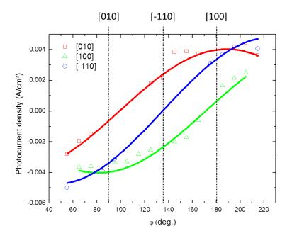
Figure 2.14: Measured photocurrent density versus crystallographic angle for three directions of light polarization. A rotation of 90° of the incident light polarization leads to a shift of 90° of the maximal photocurrent. Lines are the data fitted with the formula described in the following part of this section.
