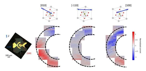
Figure 2.12: Spatially resolved photocurrent images in the circular shape electrodes gap (each frame corresponds to a full scan). Above each set of measurements the schematic orientation of the linearly polarized incident light is represented with respect to the  $BiFeO_3$  pseudocubic unit cell. The measured current is modulated by the incident polarized light and the crystallographic direction.
