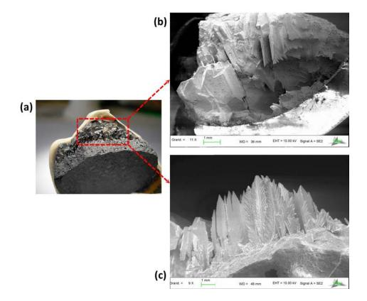
Figure 1.25: (a) Optical image of a broken crucible. Red dash square indicates a cavity where crystals have grown. (b) MEB image of as grown crystals in the cavity. (c) MEB image of dendritic shape crystals. Crystals present an unusable rough face (middle of the image) and a smooth face (left of the image) which can be used for measurements.
