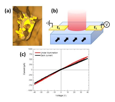
Figure 2.20: a) Single domain crystal of  $BiFeO_3$  with Au electrodes deposited on top. b) Schematics of the measurement geometry where the laser light is shun in between the electrodes. c) The I(V) curves measured in the dark and under illumination show a small photoconductance with negligible zero voltage photocurrent.
