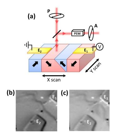
Figure 2.24: Schematics of the optical measurement where a focused laser spot is scanned on the sample and two quantities are recorded including the change of light polarization and the current extracted through the electrodes. The latter allows to map the photocurrent generation while the former gives the ferroelectric domain configuration as shown on the two images where the dark line corresponds to the domain wall.
