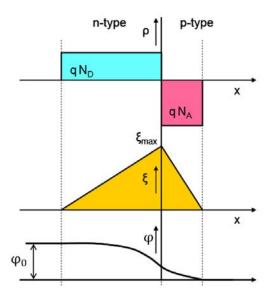
Figure 2.2: Schematics of the electric potential  $\varphi$ , electric field  $\xi$  and net charges  $\rho$  profiles in the depletion region of a pn junction.  $\varphi_0$  is the voltage resulting from the imbalance of net charges at both side of the interface.
