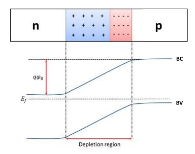
Figure 2.1: Schematics of a pn junction with its associated energy band diagram.  $\varphi_0$  is the voltage resulting from the imbalance of net charges at both side of the interface and  $E_f$  the fermi level.
