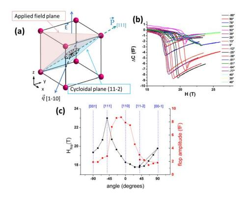
Figure 4.2: a) Geometry of the measurement where the field was rotated in the plane containing P[111] and the [001] direction (=90°) along which the capacitance is measured. b) High field measurements of the capacitance (along [001]) of a single polarization domain crystal as a function of the field direction. c) Summary of the flop fields and the amplitude of the capacitance jump amplitude as a function of angle in the measuring plane.
