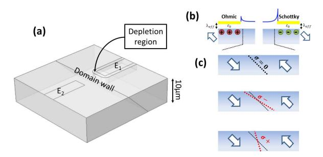
Figure 2.26: Schematics of : (a) The 3D model used for finite element calculations of the internal electric field. (b) A side view of the sample where the main boundary conditions are represented. (c) The domain wall charge depending on the angle between P and the normal to the domain wall.
