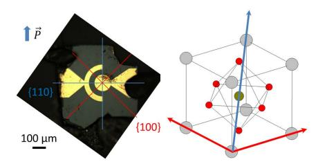
Figure 2.10: Microscope image of the  $BiFeO_3$  single crystal (001) surface with two circular shape electrodes. The main crystallographic directions are indicated as they are projected on the surface. The projection of **P** is along the [110] direction. On the right, these main directions are located in the pseudocubic unit cell.
