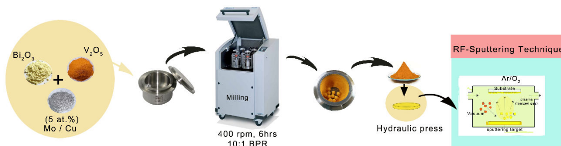
Fig.2.5. Schematic representation (work flow) for the preparation of doped \text{BiVO}_4 powders by HEM and pellet preparation and to thin films deposition by rf-sputtering technique.
