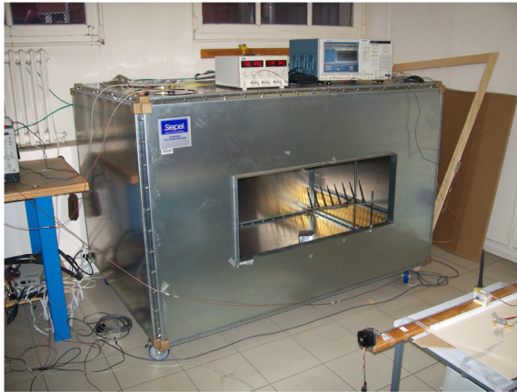
(a) Picture of the reverberation cavity
