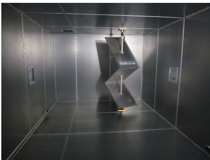
Figure 2.1 Photography of an empty Reverberation Chamber. On the left side is the vertical Mode Stirrer (or Tuner), that changes the electromagnetic boundaries ensuring a (statistically) homogeneous field distribution.
