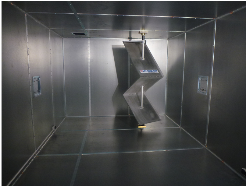
Figure 2.1 Photography of an empty Reverberation Chamber. On the left side is the vertical Mode Stirrer (or Tuner), that changes the electromagnetic boundaries ensuring a (statistically) homogeneous field distribution.
