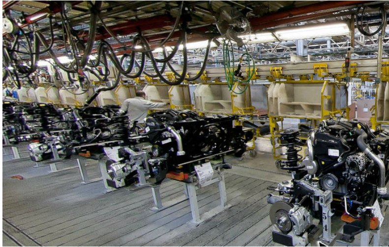
Figure 5.3 – Assemblage du GMP
