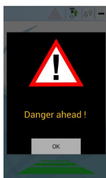
FIGURE 3.8 – Application Co-Drive qui affiche les messages d'alertes DENM
