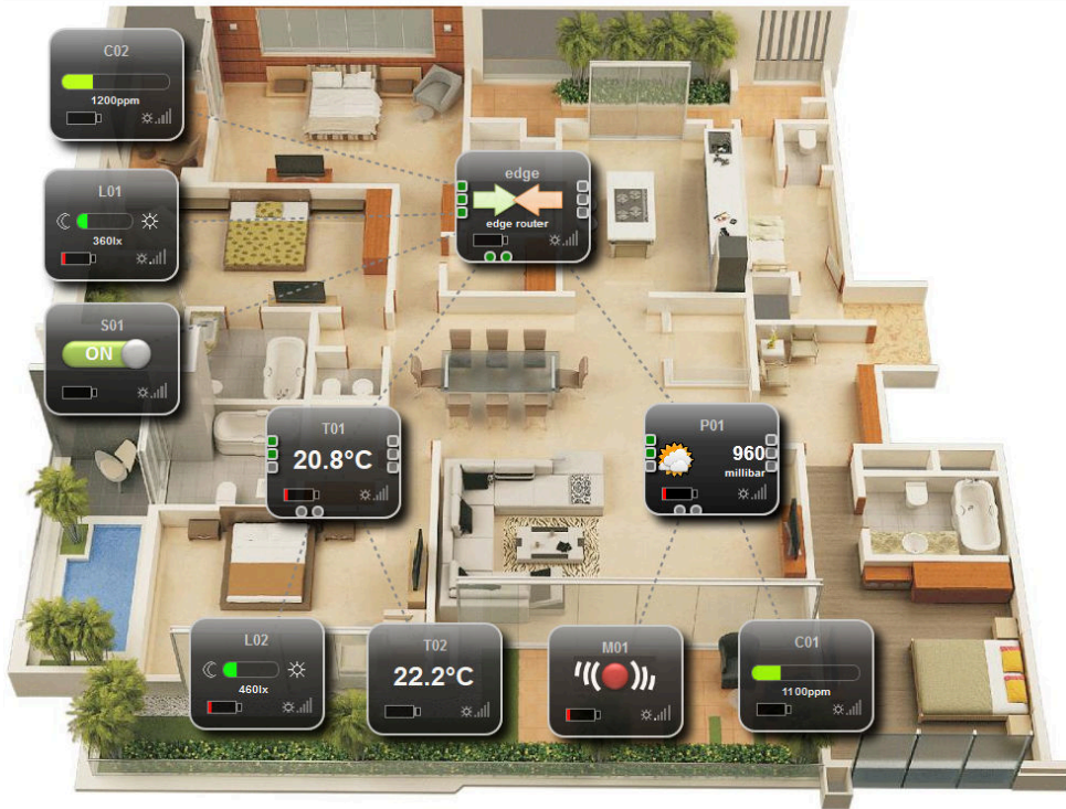
Figure 1.3: Graphical User Interface of GREENNET network
