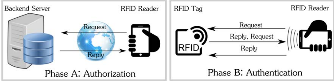
FIGURE 4.1 - The communication phases for the proposed serverless RFID authentication protocol
