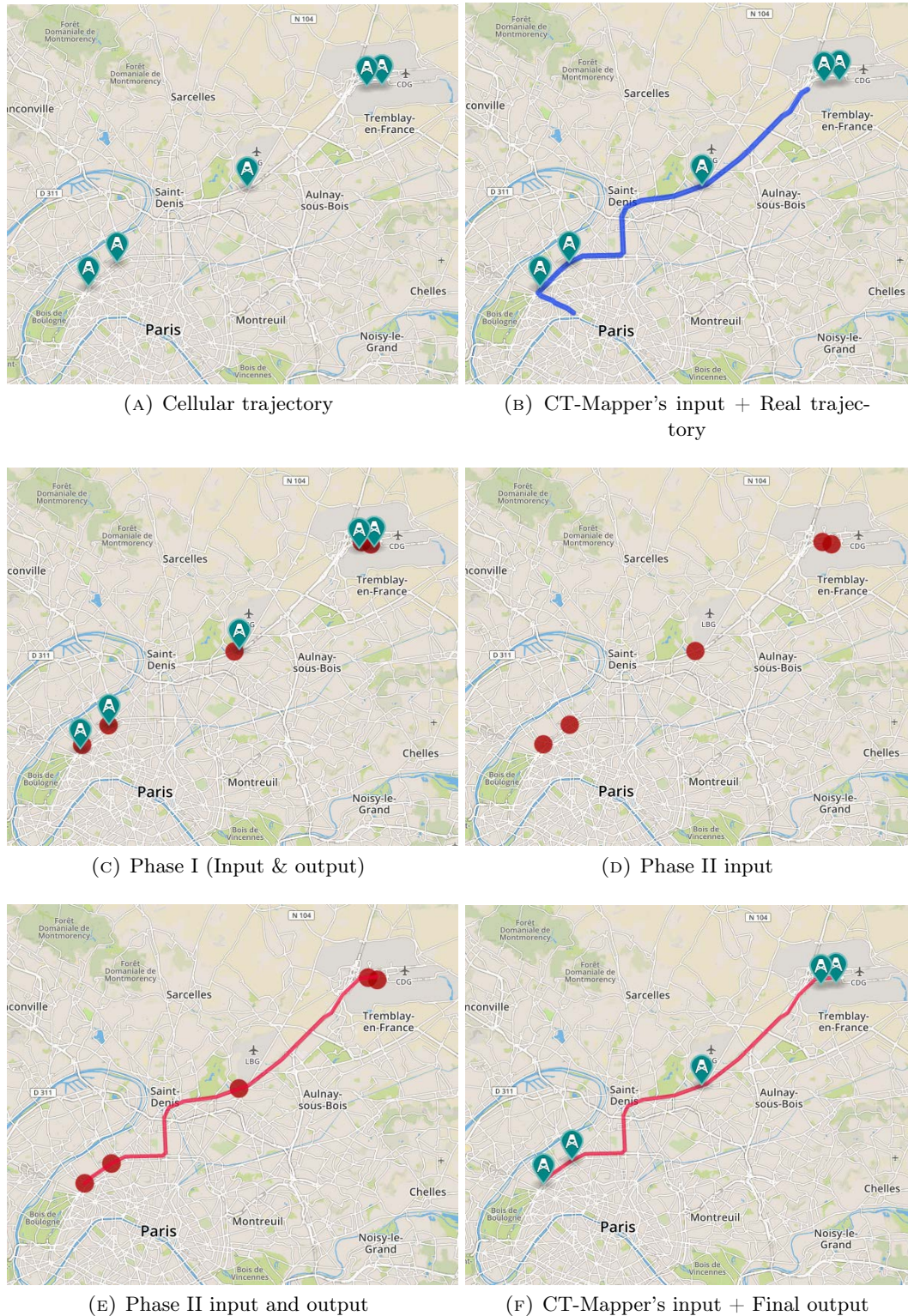
FIGURE 4.5: An illustration of different phases of mapping algorithm. The Blue line in the Fig. 5(a) is the real GPS trajectory of a user and given a sequence of 5 antenna base stations with the frequency of 15 min, the mapping algorithm can retrieve the pink line in Fig.5(e)
