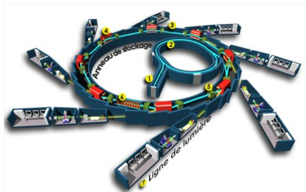
Figure 6: Scheme of a synchrotron facility. (1) LINAC, (2) Booster, (3) storage ring, (4-5) wiggler, (6) insertion device, (7) beamline.
