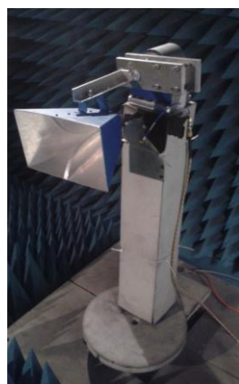
Figure 5.8 : Antenne de calibration.
