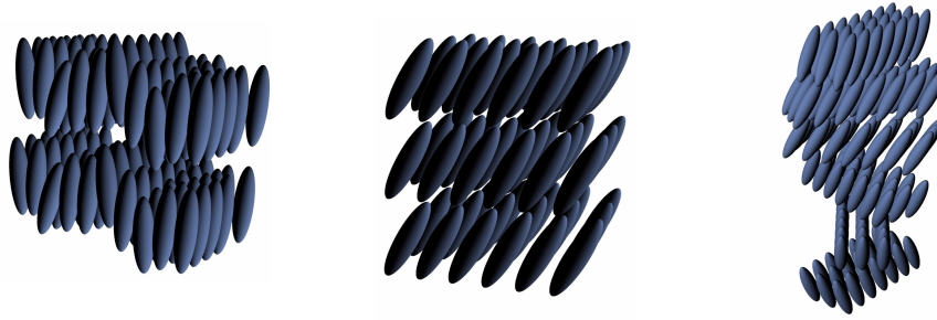
Figure 2.2: The smectic state of liquid crystal: starting from the left-hand side, smectic A, smectic C and smectic C* mesophases, respectively.
