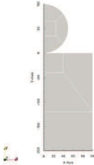
FIGURE 5.5 – Contact de Hertz, configuration en 2D
