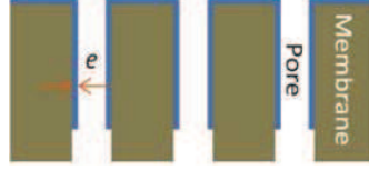
Figure 3.9: Schematic representation of pore size reduction after the photografting: polyRTIL layer in blue and support membrane in gray, e representing the graft layer thickness.
