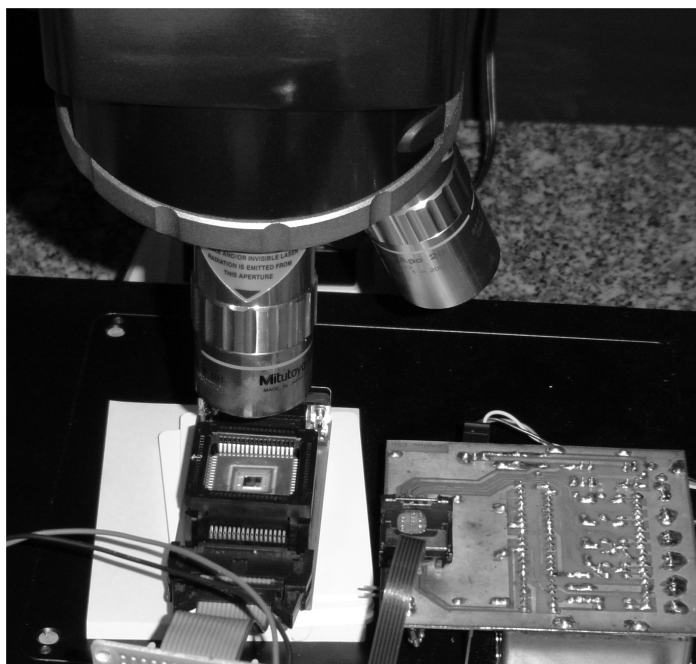
Fig. 4. Laser Fault Injection Equipment (Inner View)
