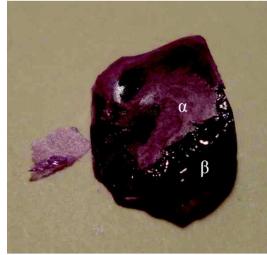
Figure 6. Thermally treated sample of Nd-metaborate glass at 754°C for 15 min showing that crystallization only starts from the surface ( \alpha : crystal layer; \beta : glass)
