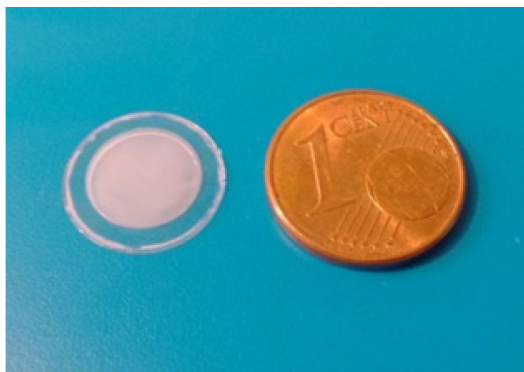
Fig. 4.5 Photograph of a 9 mm diameter PEGDA filter mounted with PEGDA ring aside a 1 cent euro coin.
