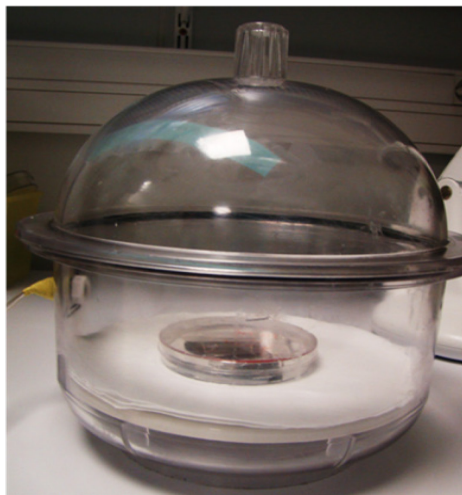
Fig. 2.11 Photograph of PDMS degassing vacuum chamber in ENS lab.
