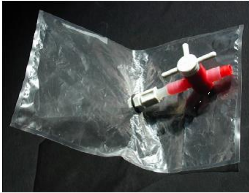
Fig. 2. 13: Tedlar bag for transportation and administration of hyperpolarized helium-3. It is closed by a non-magnetic valve.
