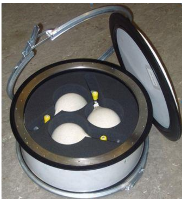
Fig. 2. 10: Transport spin box , containing three glass cells of hyperpolarized gas at 3 bar.
