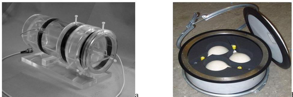
Fig.4. 2 (a) Home-made double bracelet Helmholtz RF coil used for hyperpolarized helium-3 experiments at  $f_0 \approx 48.6$  MHz. (b) Glass cells of 1 L at 3 bar pressure in the transport box where a homogenous permanent magnetic field preserves the gas hyperpolarization.
