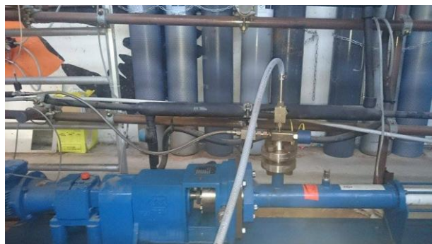
Figure II.3 – Moineau® pump (PCM Instruction Manual).
