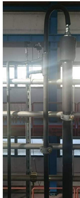
Figure II.4 – Gas separator (a) scheme (red circle: gas; blue hexagon: water) and (b) installed at the flow loop.
