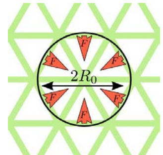
Figure 5.12: Plucking forces applied as a circular dipole of radius R_0 . The force F is counted positive if going outwards ( i.e. , an extensile dipole) and negative for a contractile dipole, as depicted here.
