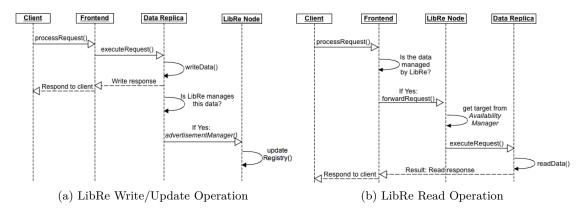
FIGURE 3.4 – Sequence Diagram of DHT-based LibRe
