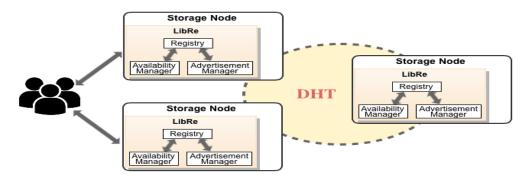
FIGURE 3.3 – Architecture Diagram of DHT-based LibRe
