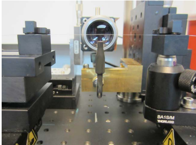
Figure 1.12: Center of the flame brushing setup. On this picture, the flame, the "V-groove" fiber clamps, the translation stages and a microscope objective are visible. The microscope objective is used for example for checking the fiber cleanliness before pulling, or for precise positioning of the torch tip.
