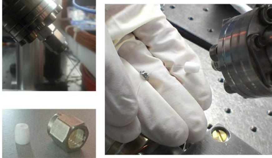
(a) Fiber feedthrough images. Top-left: the whole tightened feedthrough. Bottom left: the Teflon part and the nut. Right: all the feedthrough elements except the nut ready for assembling.
