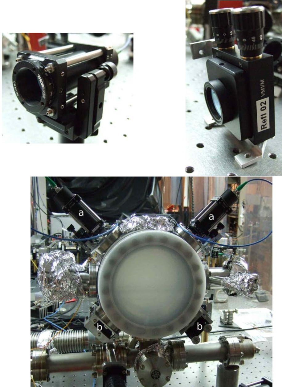
Figure 2.8: Collimation (top-left and bottom a ) and retro-reflection packages (top-right and bottom b ) for the MOT beams. The collimation package is composed of a fiber connector, a lens and a quarter waveplate. The retro-reflection package is composed of a quarter waveplate and a mirror. Both are on orientable mounts.
